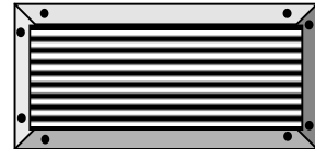
Safety mat attached to floor with aluminium extrusions
